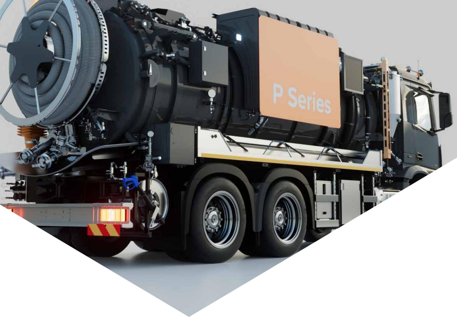
The new P series is specially designed for the professional cleaning of sewer openings and manholes.
