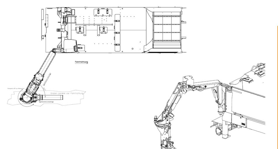
The new swivel joint increases the suction excavator's range of operation and use.
