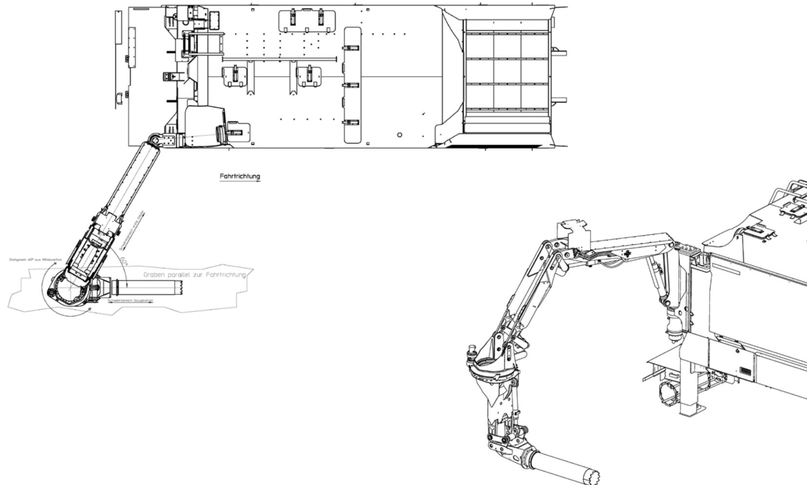
The new swivel joint increases the suction excavator's range of operation and use.
